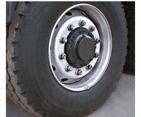
Front axle with hydrostatic wheel hub motors.
